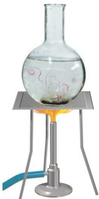
Fig. 4.9 Convection of heat in water
