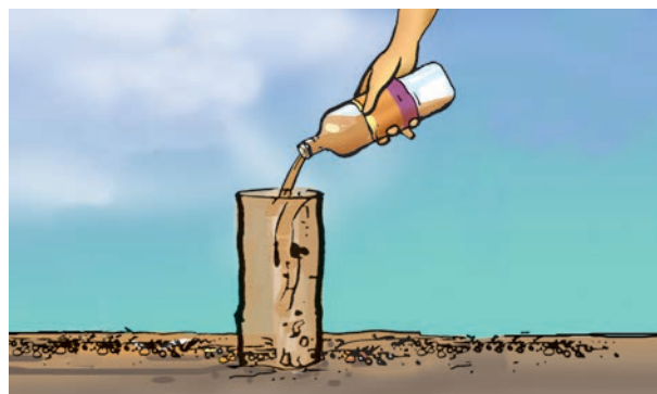
Fig. 9.5 Measuring rate of percolation
