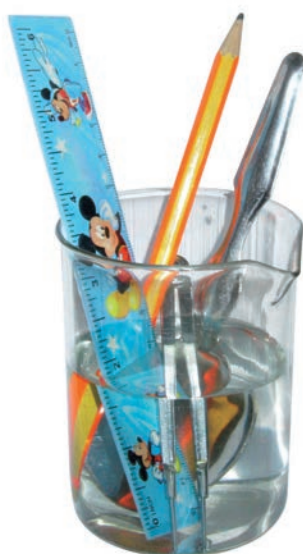
Fig. 4.8 Conduction of heat by different materials
