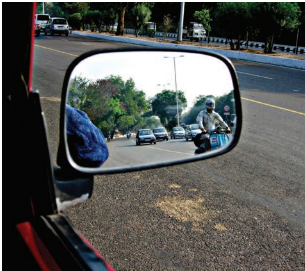
Fig. 15.20 Convex mirror as side view mirror
