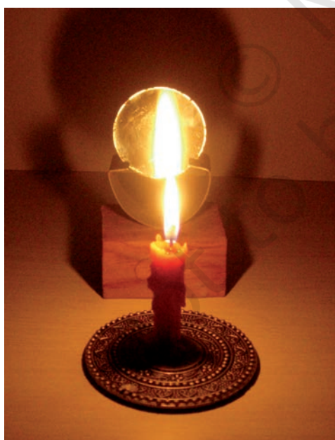
Fig. 15.16 Virtual image formed by a concave mirror
