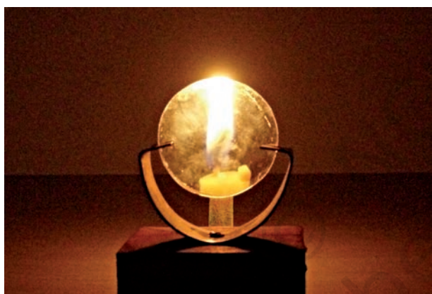
Fig. 15.26 Virtual image formed by the convex lens
