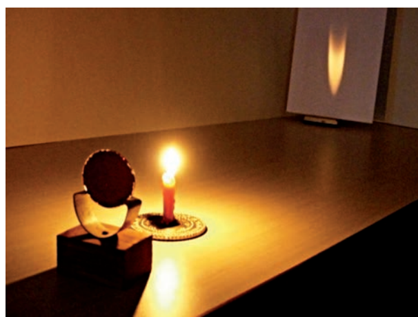
Fig. 15.15 Real images formed by a concave mirror
